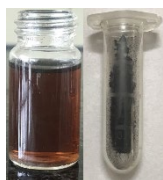
Figure 7 Liquid (left) and solid (right) samples of Nano Silver after synthesis under optimal conditions
