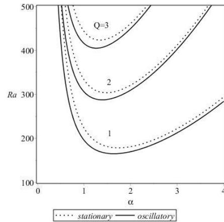
**Figure 4** Neutral stability curves of the oscillatory and stationary convection for different values of Chandrasekhar number,  $Q$  on the thermal Darcy-Rayleigh number,  $Ra$  as function of  $\alpha$  when  $Le = 1, Rn = 2, N_A = 2, \Lambda_1 = 1, \Lambda_2 = 0.5$  and  $M = 1$
