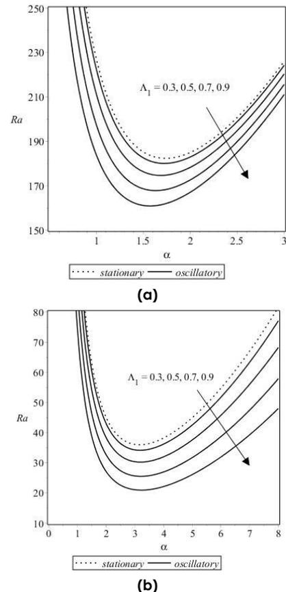
**Figure 2** Neutral stability curves of the oscillatory and stationary convection (a) with magnetic field ( $Q = 1$ ) and (b) without magnetic field ( $Q = 0$ ) for various values of scaled stress relaxation parameter,  $\Lambda_1$  on the thermal Darcy-Rayleigh number,  $Ra$  as function of  $\alpha$  when  $N_A = 2, Rn = 1, \Lambda_2 = 0.1, Le = 1$  and  $M = 1$
