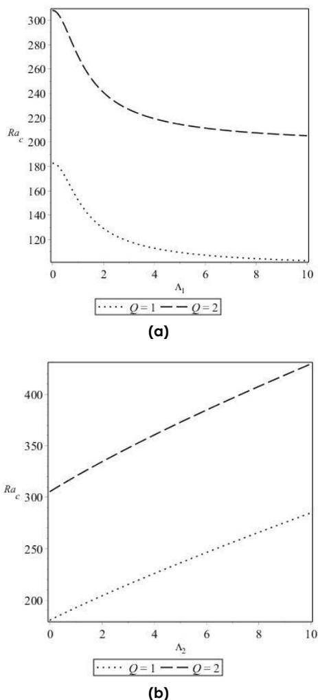
**Figure 5** The critical thermal Darcy-Rayleigh number as functions of (a)  $\Lambda_1$  and (b)  $\Lambda_2$  on the oscillatory convection for several values of  $Q$
