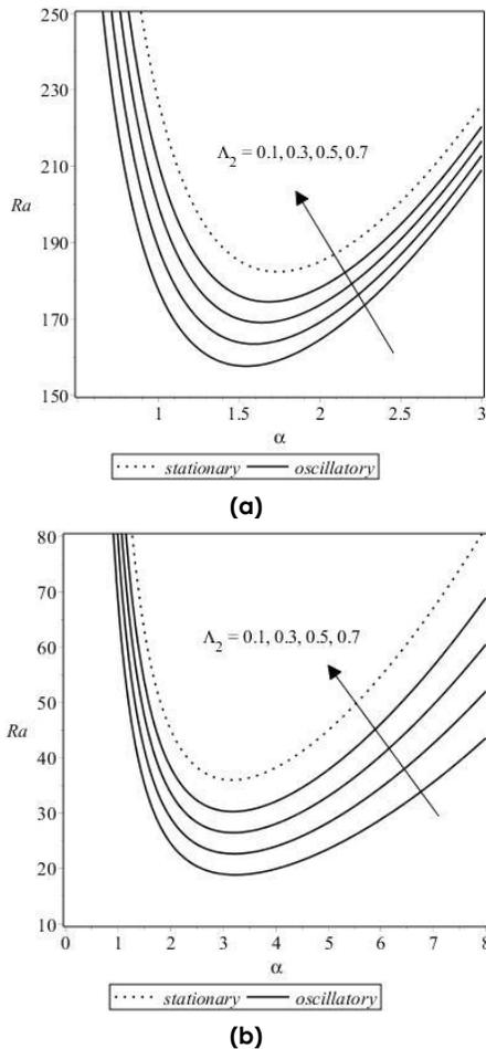
**Figure 3** Neutral stability curves of the oscillatory and stationary convection (a) with magnetic field ( $Q = 1$ ) and (b) without magnetic field ( $Q = 0$ ) for various values of scaled strain retardation parameter,  $\Lambda_2$  on the thermal Darcy-Rayleigh number,  $Ra$  as function of  $\alpha$  when  $N_A = 2, Rn = 1, \Lambda_1 = 1, Le = 1$  and  $M = 1$
