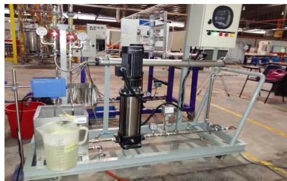
Figure 2 The pilot scale cross flow spiral wound nanofiltration set-up
