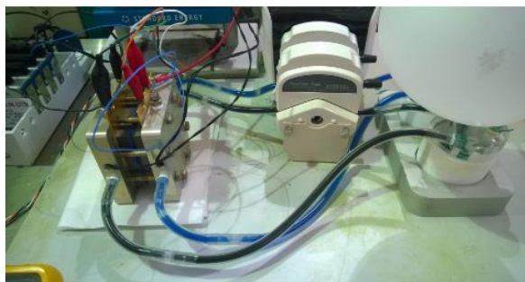
Figure 2 Photograph of VRFB single cell
