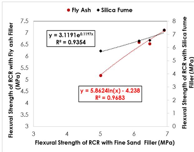
**Figure 10** Relation between 28 days flexural strength of fine sand-silica fume/fly ash minerals in RCR
