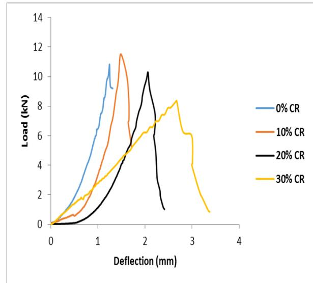
**Figure 11** Load-deflection curves for RCR with Fine sand mineral filler
