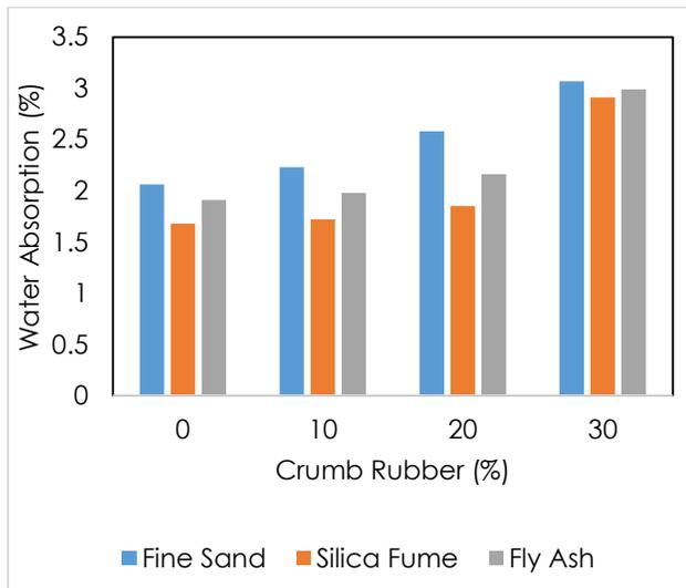
Figure 13 Water Absorption of RCR for all types of filler
