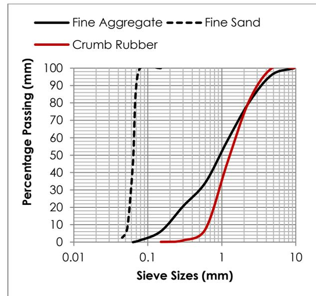
**Figure 1a** Particle size gradation of fine sand, fine aggregate and crumb rubber
