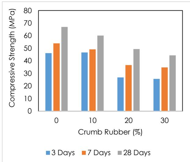
**Figure 4b** Compressive strength of RCR for silica fume mineral filler
