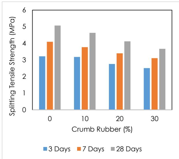
Figure 7a Splitting tensile strength of RCR for Fine sand mineral filler
