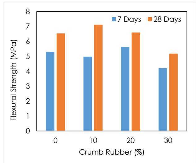
**Figure 9c** Flexural strength of RCR for fly ash mineral filler
