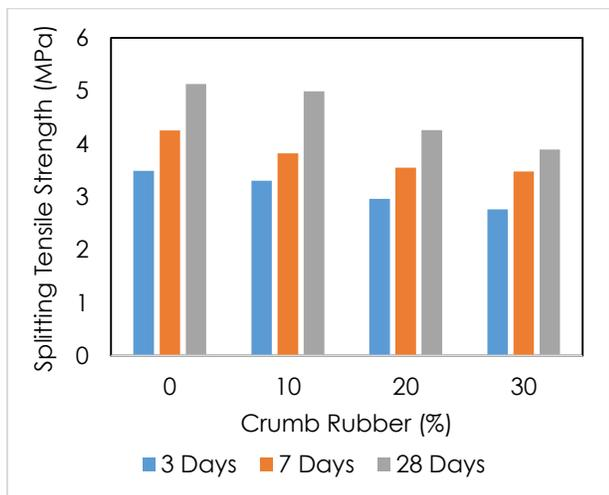
Figure 7c Splitting tensile strength of RCR for fly ash mineral filler
