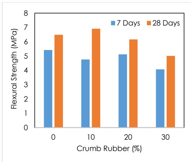
**Figure 9a** Flexural strength of RCR for natural fine sand mineral filler
