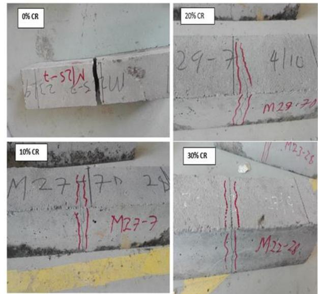
**Figure 12** Failure mode of RCR made with fine sand filler
