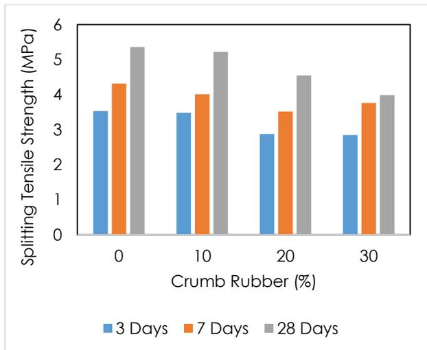
Figure 7b Splitting tensile strength of RCR for silica fume mineral filler
