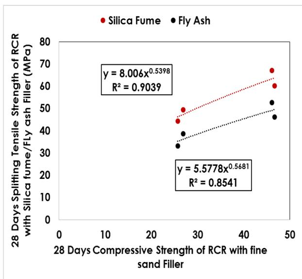
**Figure 5** Relation between 28 days compressive strength of fine sand-silica fume minerals in RCR
