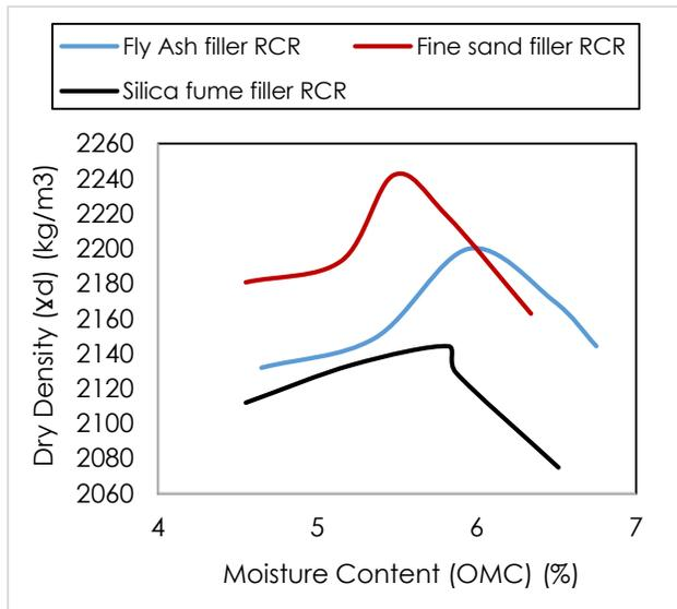
**Figure 3** Moisture content-dry density curve of RCC made with different mineral fillers
