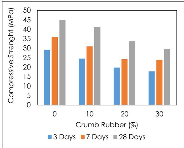
**Figure 4a** Compressive strength of RCR for natural fine sand mineral filler
