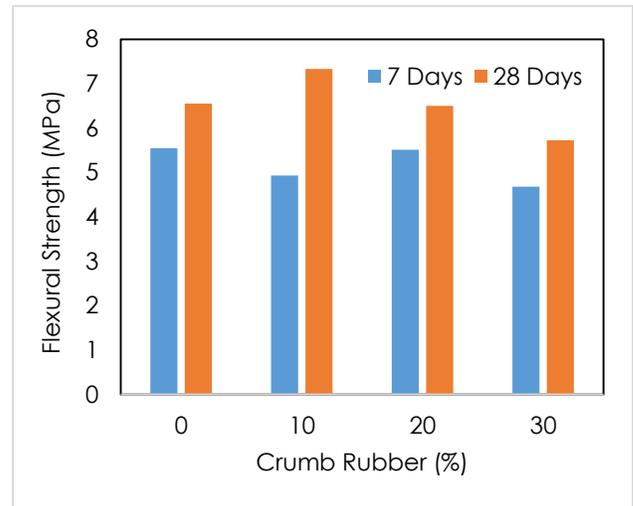
**Figure 9b** Flexural strength of RCR for silica fume mineral filler
