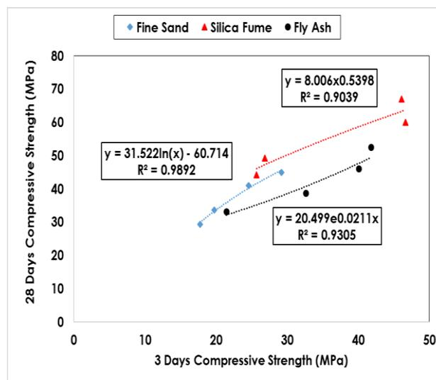
**Figure 6** Relation between 28 days and 3 days compressive strengths of RCR for all types of filler
