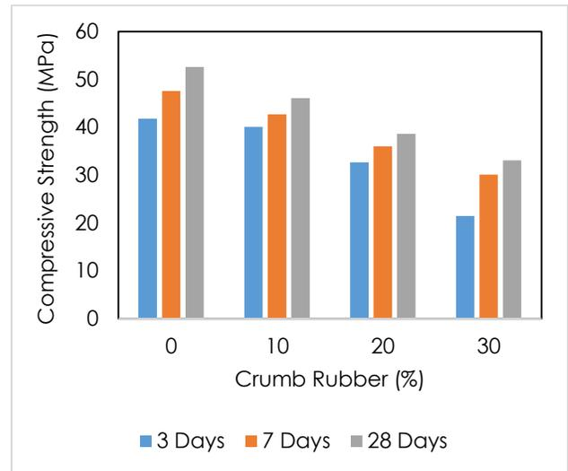
**Figure 4c** Compressive strength of RCR for silica fume mineral filler
