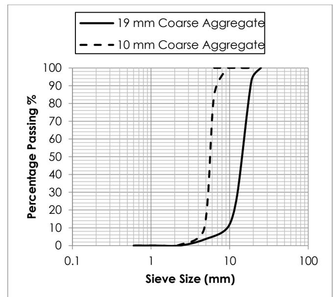
**Figure 1b** Particle size gradation of coarse aggregate
