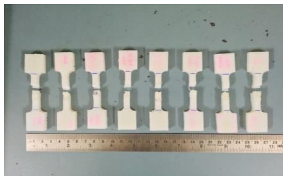
Figure 2 Sample of Fractured Specimens after Tensile Testing
