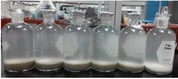
Figure 1 The settleability of ozonated sludge floc from 10 to 60 minute (left to right)
