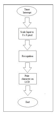
Figure 7 Flowchart of the software system
