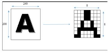
Figure 8 Scaling from the resolution of 240×200 to 8×8.
