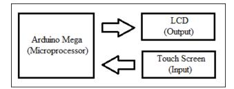
Figure 3 Basic Block Diagram of the System
