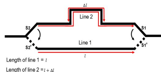
**Figure 1** Delay line concept
