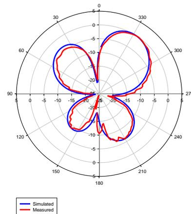
**Figure 17** Comparison of radiation pattern between Fabricated and simulated antenna at condition two (3)
