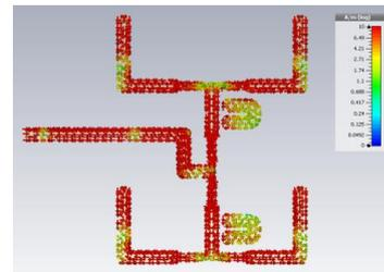
Figure 6(a) Current flow on the feeding line in condition 1
