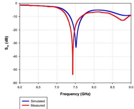
Figure 12 Comparison between Fabricated and simulated antenna at condition one (1)
