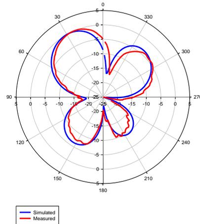
**Figure 16** Comparison of radiation pattern between Fabricated and simulated antenna at condition two (2)
