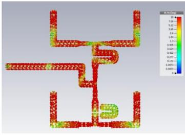
Figure 7(a) Current flow on the feeding line in condition 2
