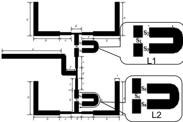
Figure 5 position of six switches and two delay lines designed on the feeding network
