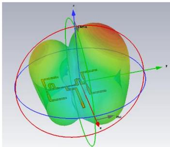
Figure 7(b) Simulation of radiation pattern in condition 2
