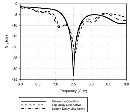
Figure 9 Values of  $S_{11}$  for three conditions of switches modes
