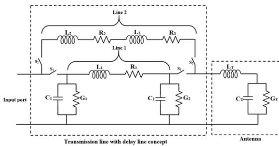
Figure 2 Equivalent circuit for the delay line concept
