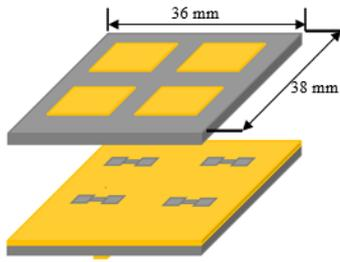
Figure 4 Two by two (2 x 2) Antenna array
