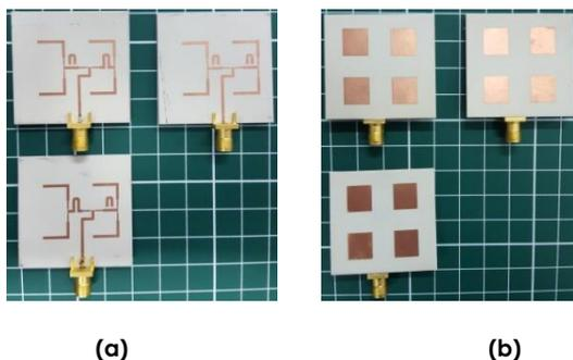
Figure 11 Fabricated antenna with different condition of feeding line, (a) Rear view, and (b) front view
