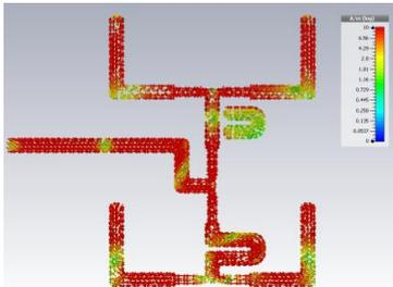
Figure 8(a) Current flow on the feeding line in condition 3
