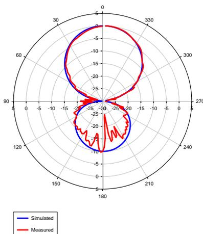
**Figure 15** Comparison of radiation pattern between Fabricated and simulated antenna at condition one (1)
