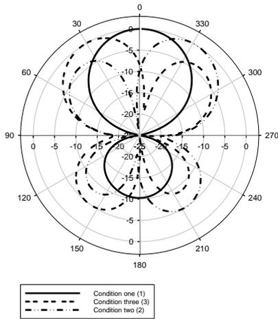
Figure 10 Radiation patterns for three different angles
