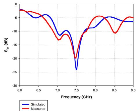
Figure 14 Comparison between Fabricated and simulated antenna at condition three (3)
