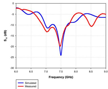
Figure 13 Comparison between Fabricated and simulated antenna at condition two (2)
