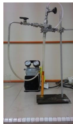
Figure 3 Vacuum deposition setup for catalyst deposition
