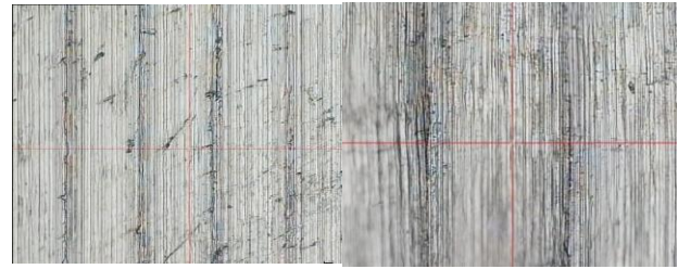
V_c = 105 m/min, f = 0,10 mm/rev V_c = 105 m/min, f = 0,15 mm/rev
