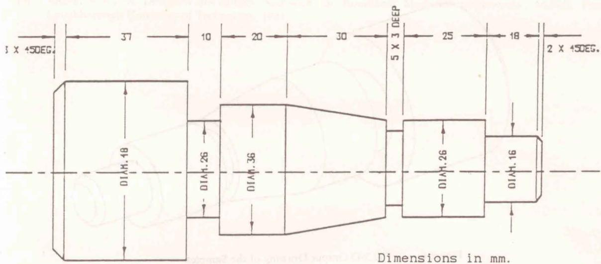
Figure 5: The Sample of the Rotational Component
