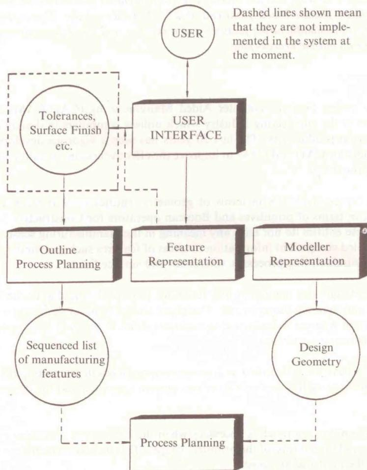
Figure 1: The Main Component of the System.
