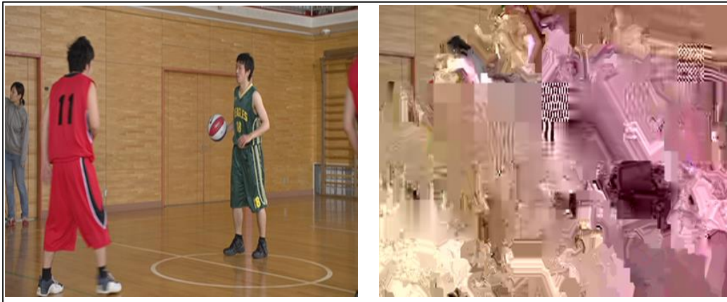
Figure 8 Key sensitivity for encrypted frame #1 of BasketBallPass video sequence, encrypted with 1-bit different key
