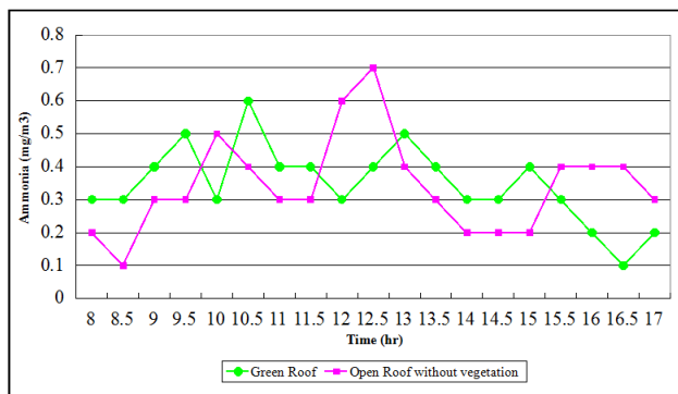
Figure 8 Ammonia content on green roof is higher than open roof
