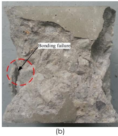
Figure 7 Failure mode of cubic specimens (a) SCLWC (b) SCC
