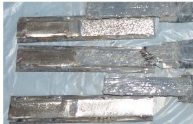
(b) CFRP rupture failure
