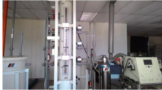
Figure 2 Hybrid Biogranular Sludge Reactor
