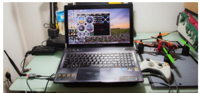
Figure 7 A UAV Quadrotor System with Notebook and Xbox joystick
