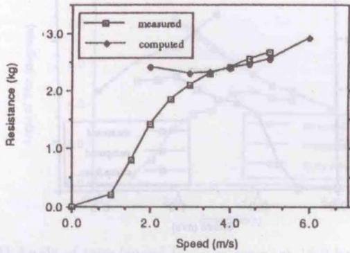
Fig. 24 Total resistance/speed for displacement 18.9 kg and leg 47.1 cm
