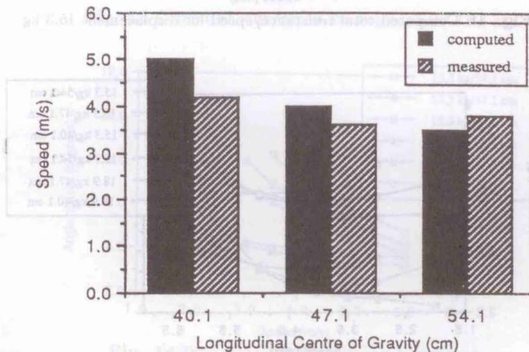
Fig. 18 Start of planing for displacement 18.9 kg
