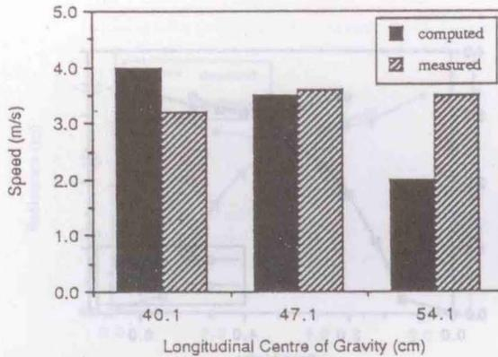
Fig. 19 Start of planing for displacement 15.3 kg
