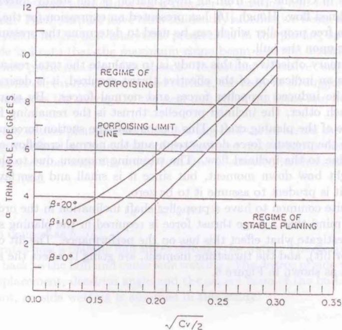
Fig. 7 Relationship between trim angle and lift coefficient [8]
