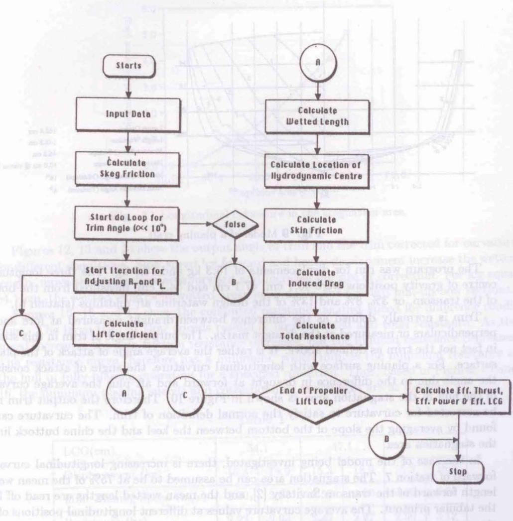
Fig. 8 Computer flowchart for resistance prediction
