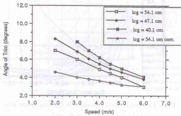
Fig. 13 Computed trim/speed for displacement 15.3 kg
