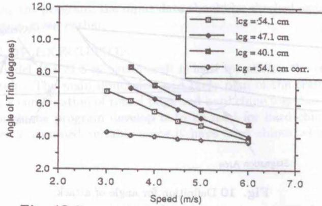
Fig. 12 Computed trim/speed for displacement 18.9 kg
