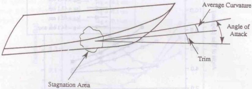
Fig. 10 Definition for angle of attack
