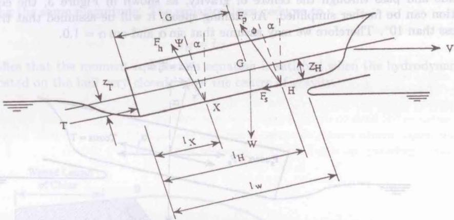
Fig. 1 Hydrodynamic and static forces on a planing hull
