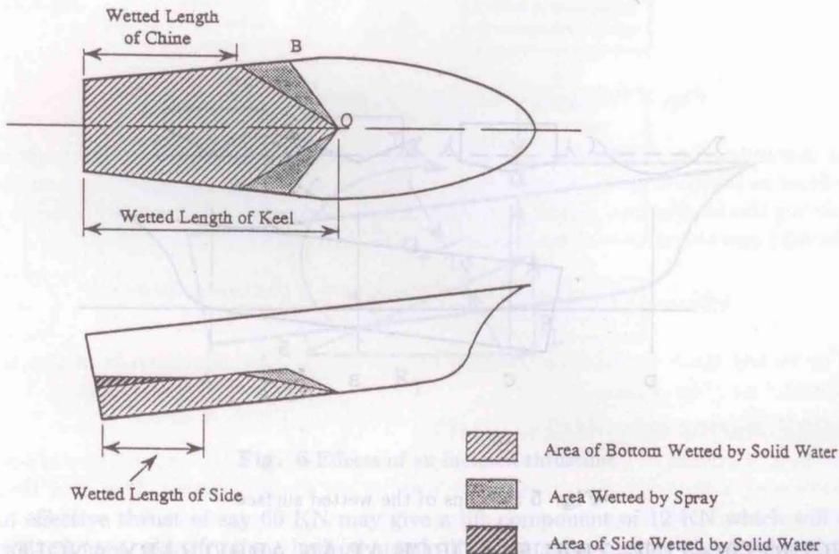
Fig. 4 Geometry of the wetted surface
