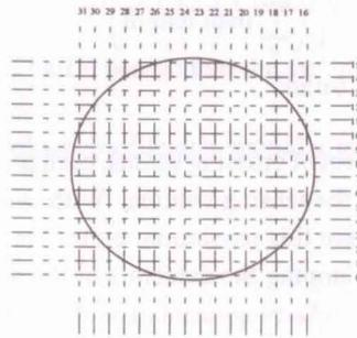
Figure 1 Arrangement of two orthogonal 16 transducer projections
