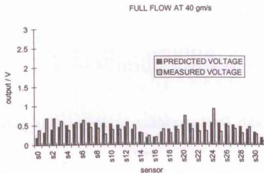
Figure 8a Full flow for plastic beads at 40 gm/s
