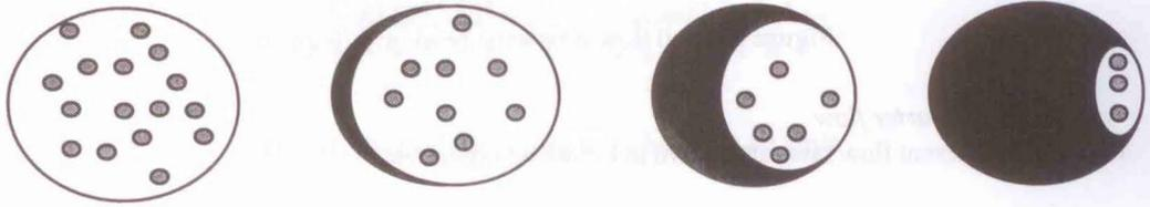
a. Full flow                      b. Three-quarter flow      c. Half flow                      d. Quarter flow
