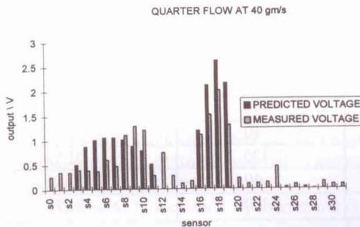
Figure 11a Quarter flow for plastic beads at 40 gm/s
