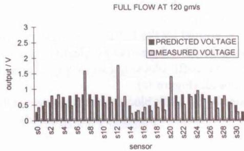
**Figure 8b** Full flow for plastic beads at 120 gm/s
