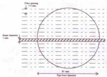
Figure 2 Dimensions of 16 transducer projection
