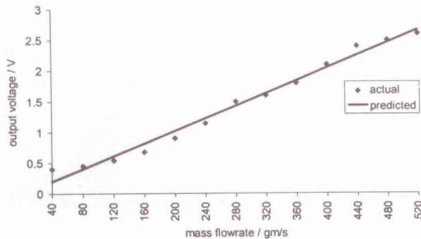
**Figure 6** Relationship between mass flow rate and optical sensor output voltage for optical fibre receiver number twenty five
