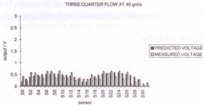
**Figure 9a** Three quarter flow for plastic beads at 40 gm/s
