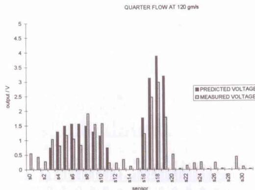
Figure 11b Quarter flow for plastic beads at 120 gm/s
