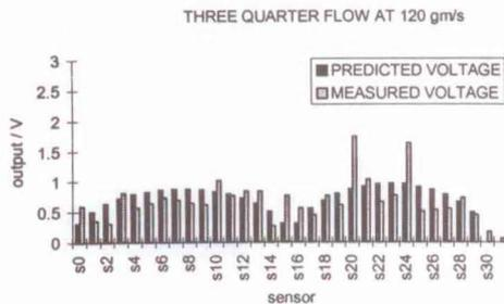
**Figure 9b** Three quarter flow for plastic beads at 120 gm/s
