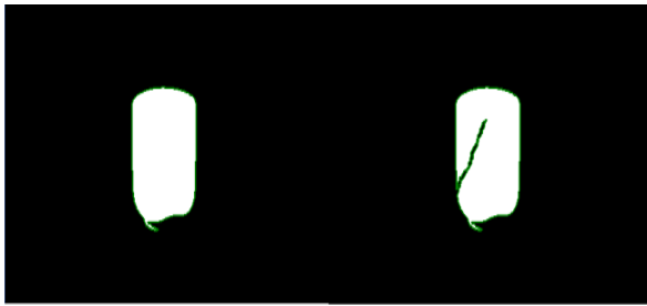
Figure 7 Threshold image of (a) good ceramic cup and (b) cracked ceramic cup
