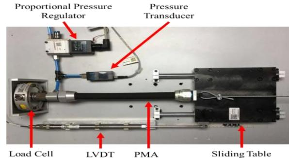
Figure 3 1-DOF horizontal PMA experimental setup
