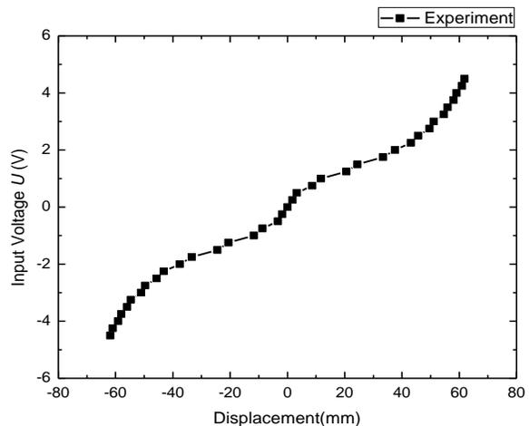
Figure 7 Feedforward element – relationship between the displacement and input voltage
