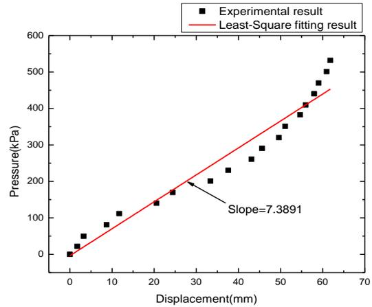
Figure 5 Pressure – Displacement nonlinear function
