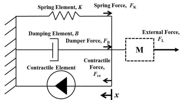
Figure 2 Three element phenomenological model of PMA
