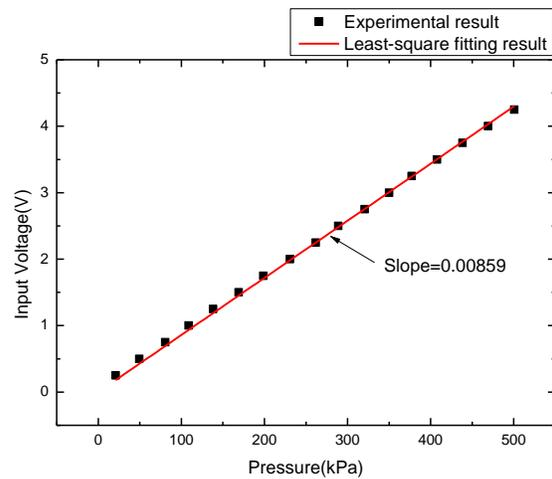
Figure 6 Linearizer – relationship between the pressure and input voltage
