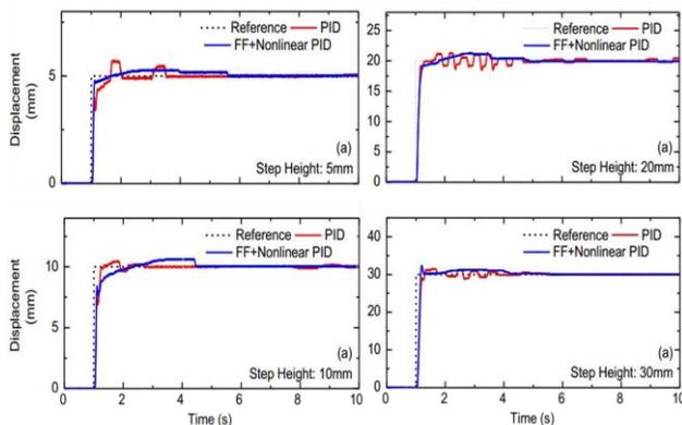
**Figure 9** Experimental positioning responses to different step heights in the presence of mass change
