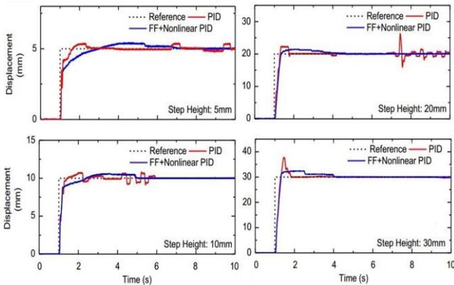
**Figure 8** Experimental positioning responses to different step heights with default mass
