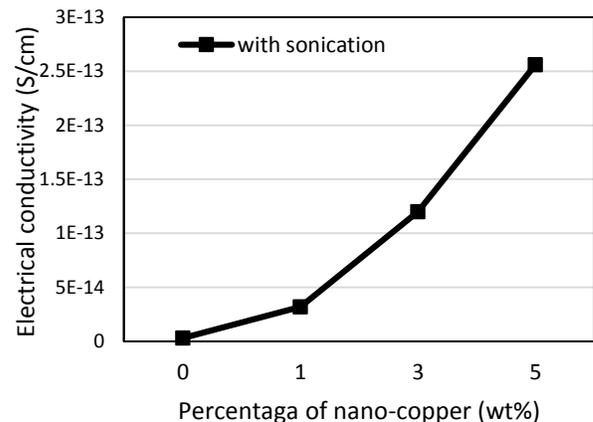
**Figure 6** Electrical conductivity of nylon 66/nano-copper nanocomposite with sonication
