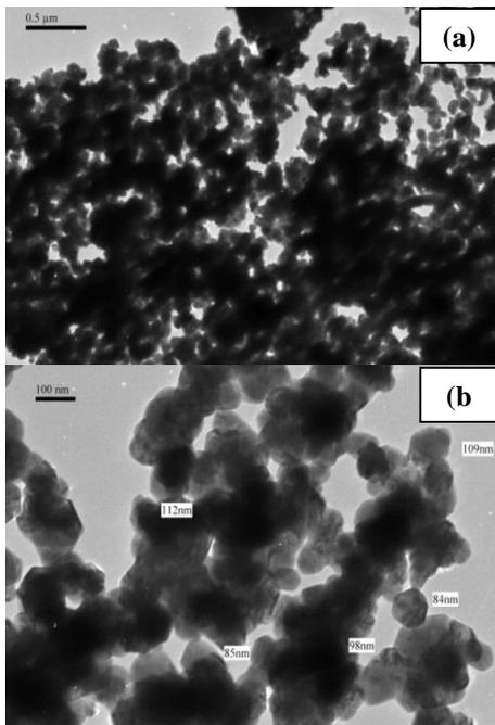
**Figure 1** Nano-copper dispersion in ethanol solution without sonication at (a) 6,000X magnification and (b) 20,000X magnification
