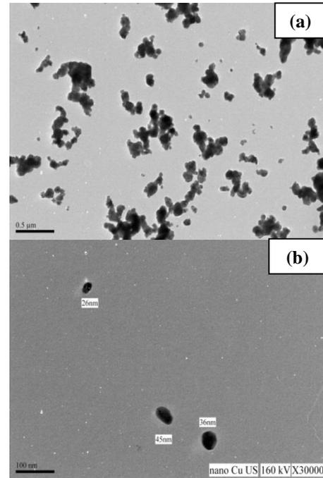
**Figure 2** Nano-copper dispersion in ethanol solution with sonication at (a) 6,000X magnification and (b) 30,000X magnification
