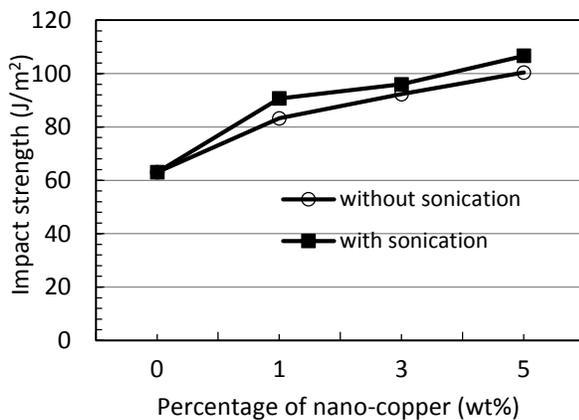
**Figure 4** Impact strength of nylon 66/nano-copper nanocomposite containing various amount of nano-copper
