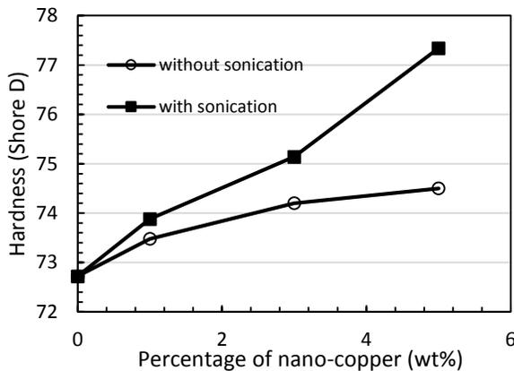
**Figure 3** Hardness of nylon 66/nano-copper nanocomposite containing various amount of nano-copper
