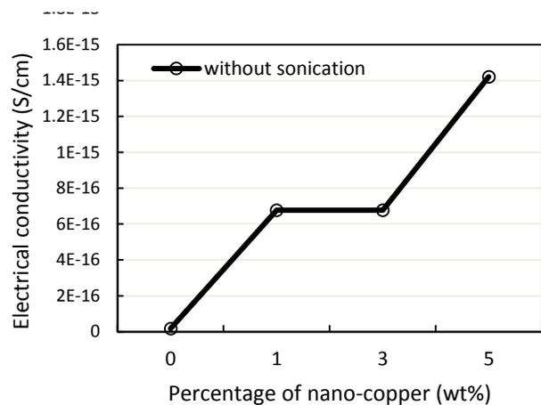
**Figure 5** Electrical conductivity of nylon 66/nano-copper nanocomposite without sonication
