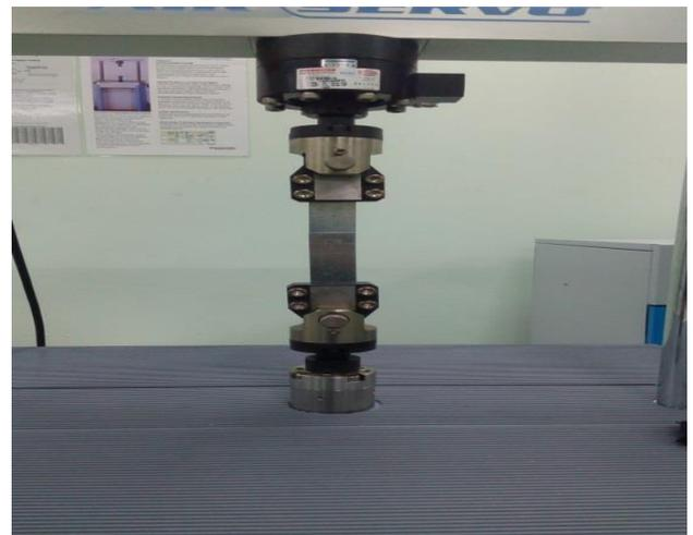
Figure 3 The mounting specimen with the jig
