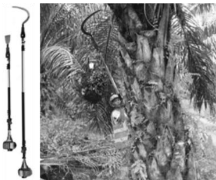
Figure 2 Harvesting oil palm FFB with Cantas sickle (Source: http://www.palmeka.com )
