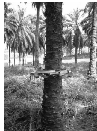
Figure 9 Climbing robot with tilt sensors (Source: Shokripour, et al., 2010)
