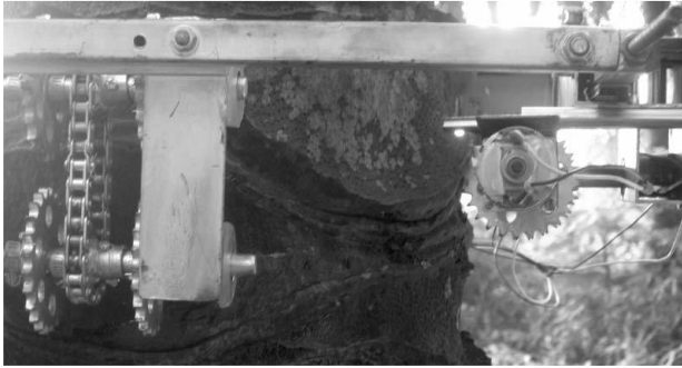
Figure 10 Robot climbing smooth trunk using small sprockets (Source: Shokripour, et al., 2010)
