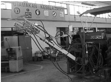
Figure 5 Wire cutting mechanism mounted on tractor (Source: Wan Ismail, 2010)
