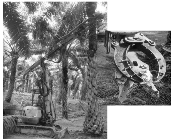
Figure 8 Track-type harvesting machine for tall trees (Source: Shuib, et al., 2004)
