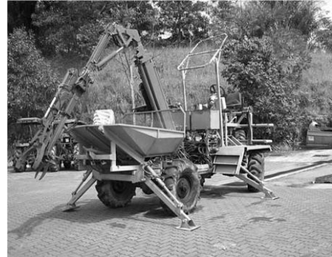
Figure 7 MPOB-UPM's wheel-type mechanical harvesting machine (Source: Shuib, et al., 2011)
