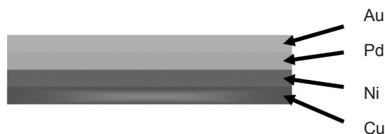
Figure 1 The deposition layers of ENEPIG surface finish
