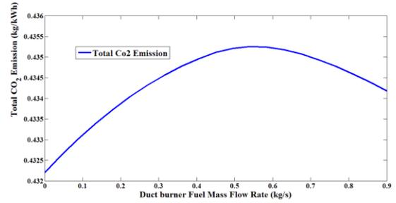
**Figure 6** Effect of DB fuel flow rate on CO<sub>2</sub> emission of the plant
