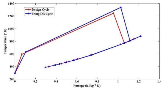
**Figure 7** Comparing gas turbine cycle for both cycles in T-S plane
