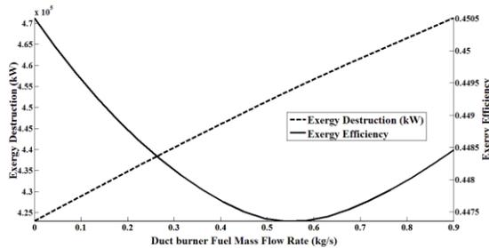
**Figure 5** Effect of DB fuel flow rate on exergy efficiency and exergy destruction of plant
