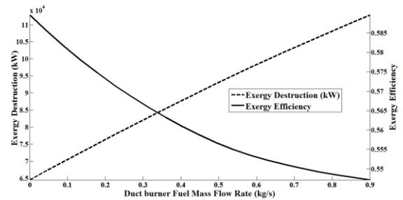
Figure 3 Effect of DB fuel flow rate on the exergy efficiency and exergy destruction rate of the bottoming cycle
