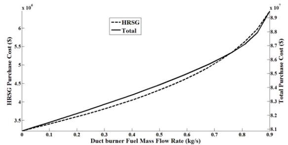
Figure 2 Effect of DB fuel flow rate on the HRSG purchase cost and total purchase cost
