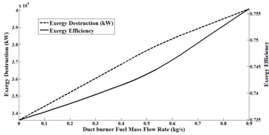
**Figure 4** Effect of DB fuel flow rate on exergy efficiency and exergy destruction of the steam cycle
