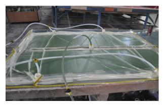
Figure 1 Vacuum bagging infusion process
