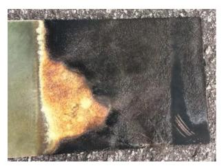
Figure 4 Delamination of fibres
