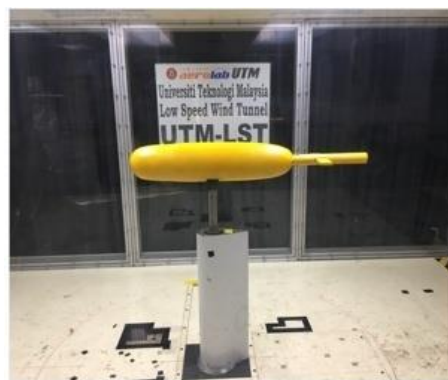
Figure 2 Ellipsoidal fuselage mated with Forward stabilizer
