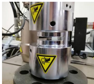
Figure 2 The specimen was placed on the load cell
