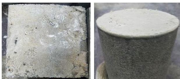
Figure 3 Collapsible foam layer
