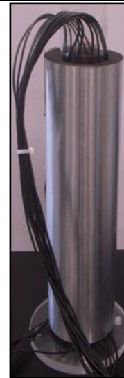
Figure 4 Dual plane ECT sensor with external shield
