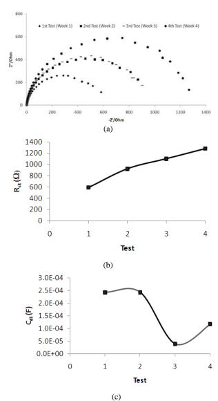
**Figure 2** a) Nyquist plot for AA5083 immersed in POME b) Plot of charge transfer resistant,  $R_{ct}$  c) Plot of double layer capacitance,  $C_{dt}$
