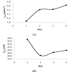
**Figure 4** a)  $I_{corr}$  and b)  $E_{corr}$  plots of AA5083 in POME
