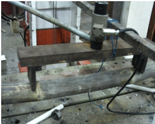
(a) Failure due to flexural load
