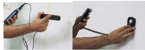
Figure 3 Calculation of the surfaces' reflectance through measuring: (left) luminance; (right) illuminance
