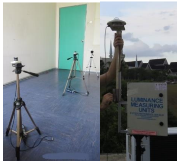
Figure 2 Measuring illuminance levels by (left) internal sensors; (right) external sensor
