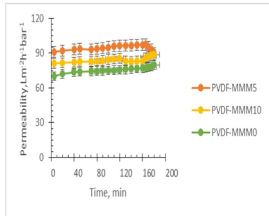
**Figure 5** Membrane permeability as the function of time
