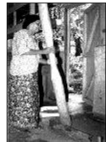
Pounding the clay using wooden hand pestle
