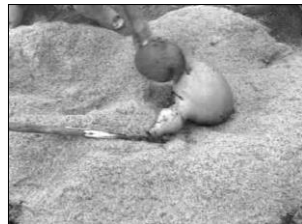
The fiery hot body is placed in a pile of paddy husks to obtain the blackened effect
