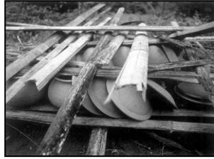
Arranging the wood & bamboo strips before firing process for Mambong
