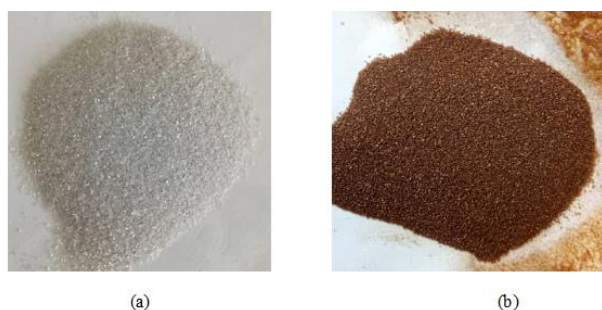
Figure 1 Photo of the sand (a) before and (b) after decorated with Fe 3 O 4 nanoparticles
