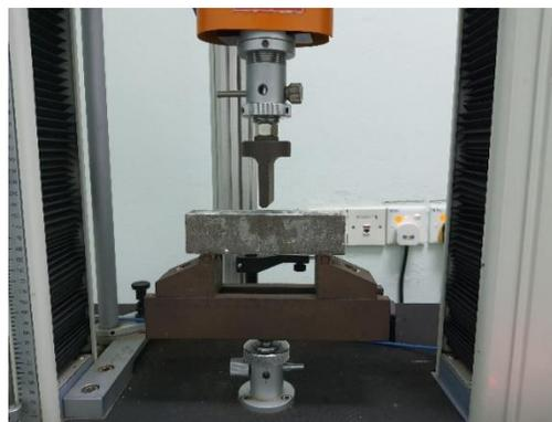
**Figure 2** Flexural strength testing using the universal testing machine
