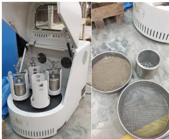
**Figure 1** Planetary grinding ball mill (left) and sieve to separate SBEA from balls (right)
