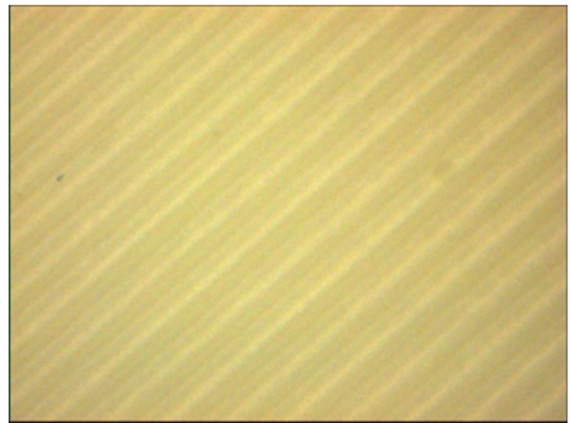
Figure 10 Printed specimen by optimal grey relational grade (GRG) setting level of printing speed (level 1), layer thickness (level 3), and surface layer (level 1)
