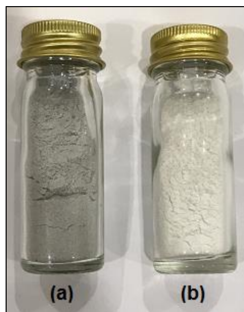
Figure 2 Appearance of RHA and RHS samples: (a) RHA extracted from untreated rice husks incinerated at 700°C; and (b) RHS extracted from solvent-thermal treated and leached rice husks in 1.0 M HCl, followed by incineration at 700°C
