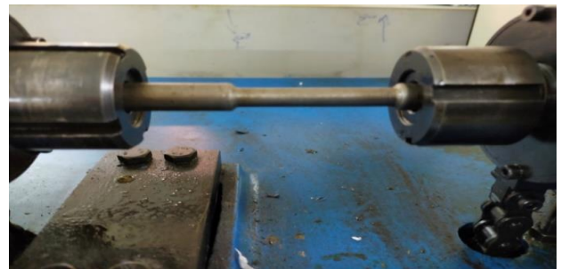
Figure 1 Dimension of the standard fatigue sample and rotating bending fatigue testing
