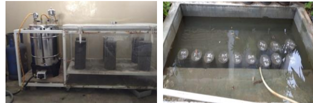
Figure 2 a. Steam Curing Process, b. Water Curing Process
