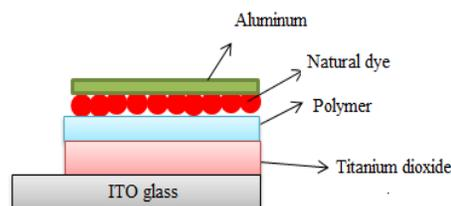
**Figure 3** Bilayer heterojunction structure of hybrid solar cells
