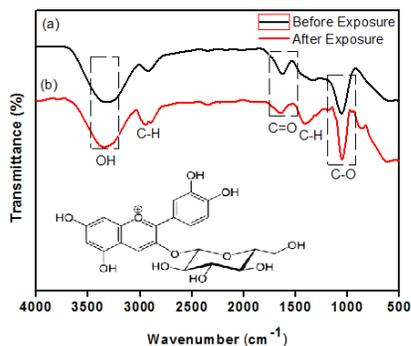
**Figure 11** FTIR *Eugenia Claviflora* before and after exposure to sunlight
