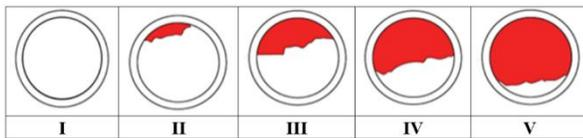
**Figure 4** Dye penetration coverage percentage scale
