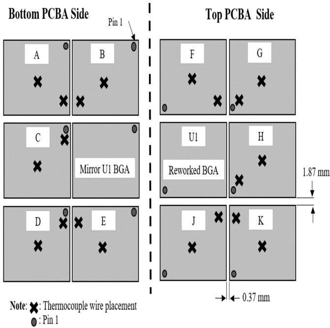
**Figure 1** Schematic of the BGA components layout and reworked component location (U1)
