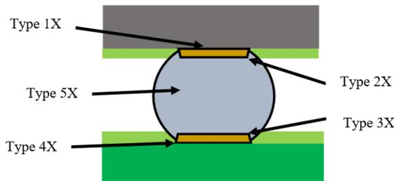
**Figure 5** Schematic of D&P separation location type
