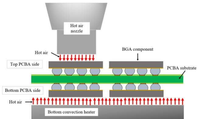
**Figure 3** Schematic of BGA component being reworked with hot air rework machine
