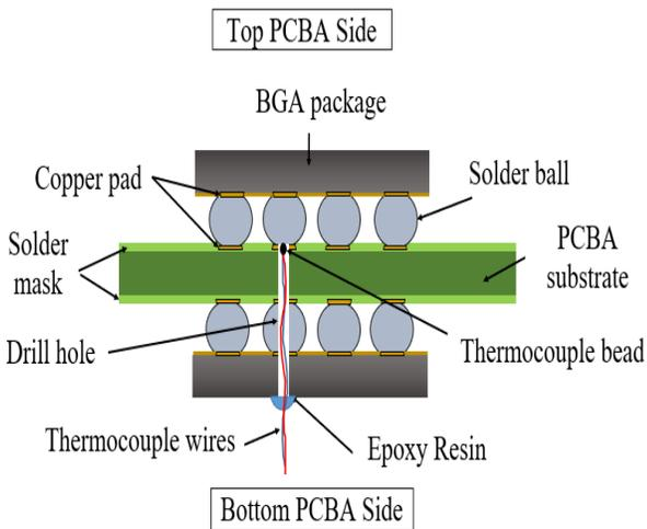
**Figure 2** Schematic of thermocouple wire location on BGA solder joint
