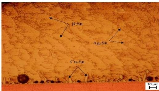
**Figure 2** Microstructure of control SAC305 solder
