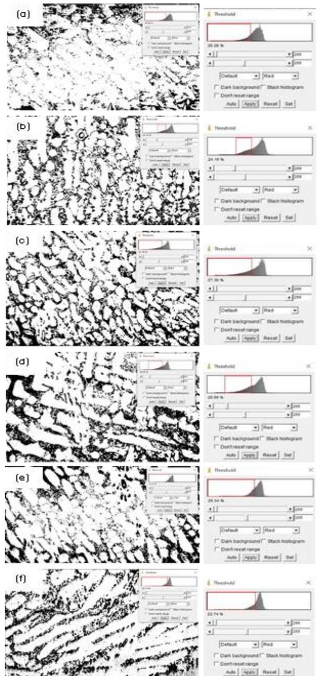
**Figure 3** The micrograph of (a) control SAC305, (b) 5 Gy, (c) 10 Gy, (d) 15 Gy, (e) 20 Gy, and (f) 25 Gy after etching
