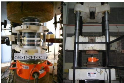
Figure 6 Diagram for strain measuring equipment and the loading device (TINIUS OLSEN Super “L” Universal Testing Machine)
