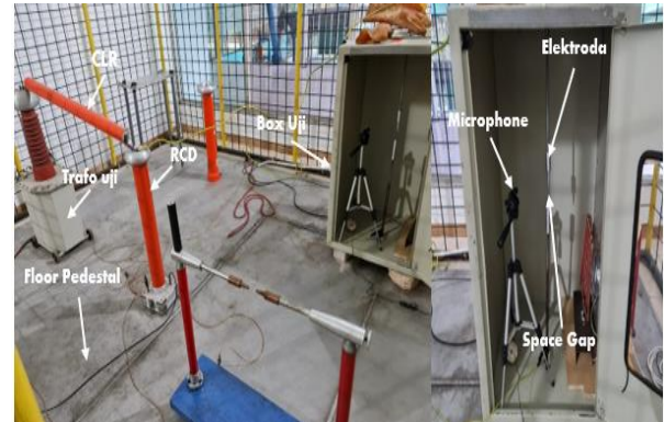
Figure 5 Research design of Corona Discharge Acoustic Recording in Cubicle 20 kV
