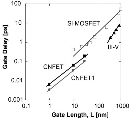
**Figure 8** Gate delay as a function of gate length
