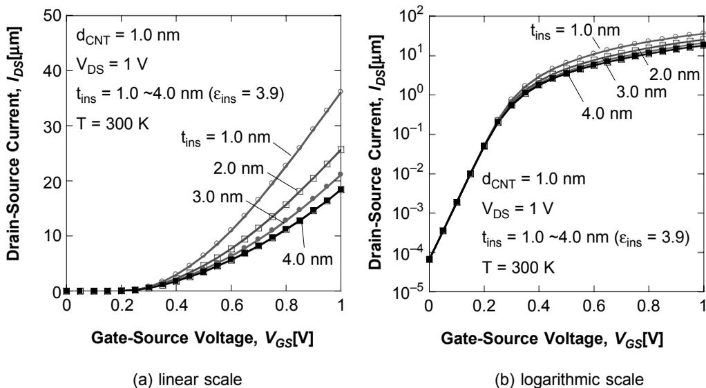
**Figure 3** Effect of insulator thickness on  $I_{DS}$  vs.  $V_{GS}$
