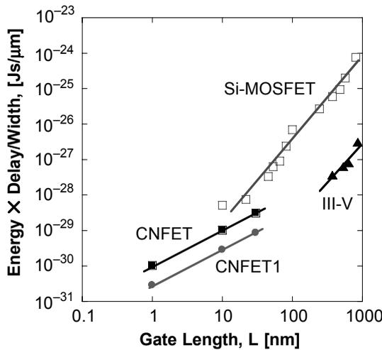
**Figure 9** Energy delay product as a function of gate length
