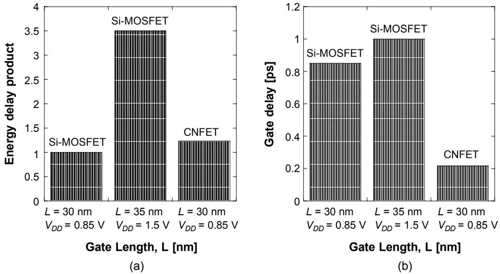
**Figure 10** Effect of drain bias on (a) EDP (b) gate delay
