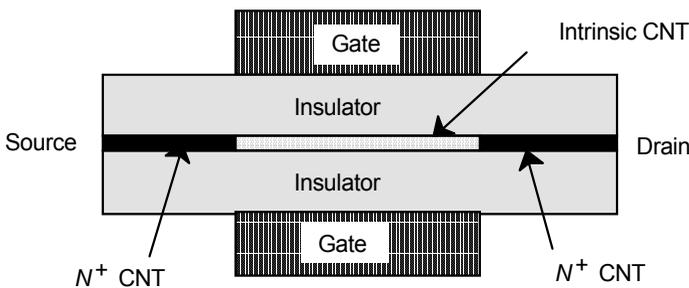
**Figure 1** Diagram of MOSFET-like CNFET
