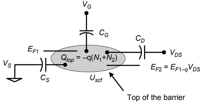
**Figure 2** The 2D MOSFET-like CNFET model used for simulation study
