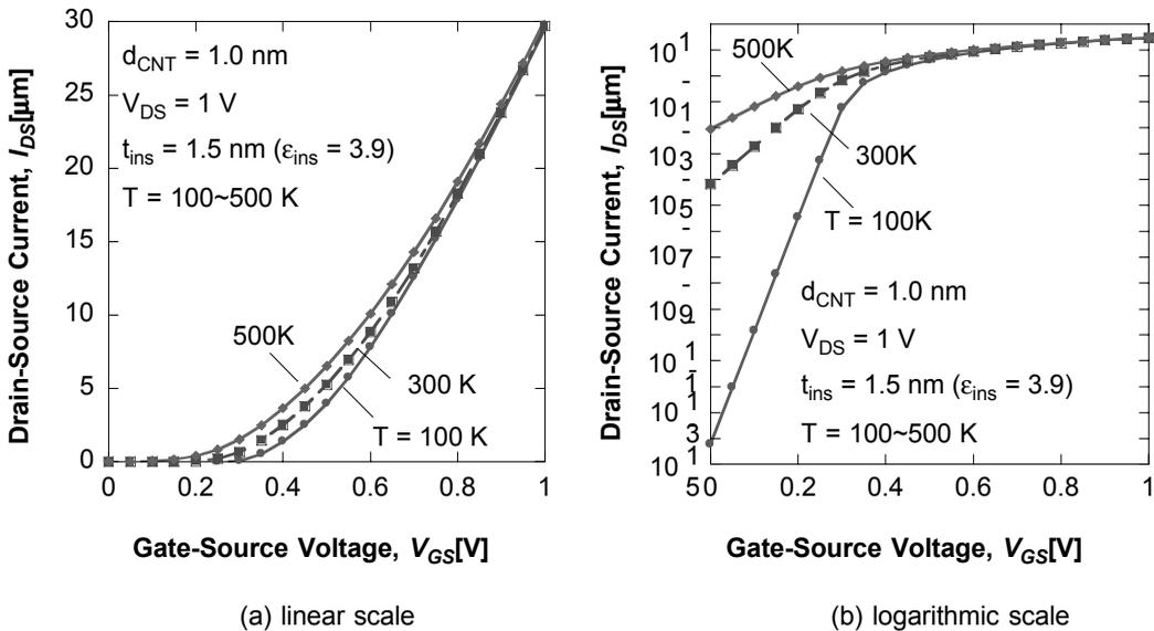
**Figure 5** Effect of temperature on  $I_{DS}$  vs.  $V_{GS}$
