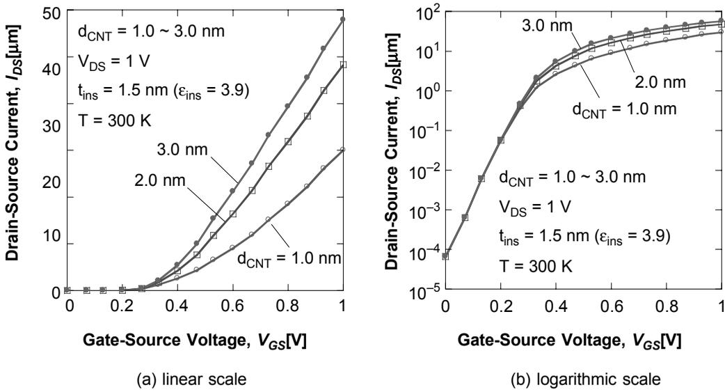
**Figure 4** Effect of CNT diameter on  $I_{DS}$  vs.  $V_{GS}$
