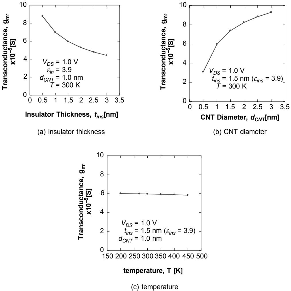
**Figure 7** Transconductance characteristics as a function of (a) insulator thickness (b) CNT diameter and (c) temperature
