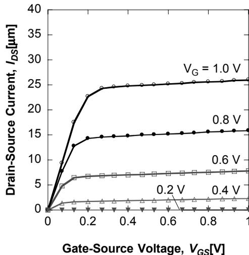
**Figure 6**  $I_{DS} - V_{DS}$  characteristics of MOSFET-like CNFET
