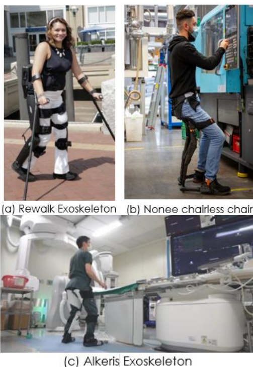
Figure 1 (a) ReWALK exoskeleton [19] for rehabilitation, (b) Nonee chairless chair exoskeleton [29] for tasks in industry, and (c) Alkeris exoskeleton [5] for surgical procedures
